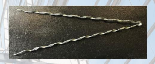
Brace ends are designed to provide fast and efficient guy strand termination in metal building construction. They are designed for use with standard guy strands 9/16 diameter or less. Holding strength is a minimum of 100% of the rated strength of the strand. Bracing ends have a left hand lay and are available in a complete range of sizes to fit any guy strand size. Birmingham Fastener's brace ends are manufactured by Payer Industries ®.
